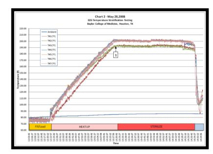
Temperature stratifications created by agitator motor failure, were quickly eliminated when the agitator motor was re-enabled.
