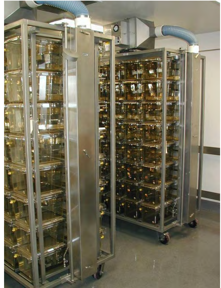
Micro Isolator racks
