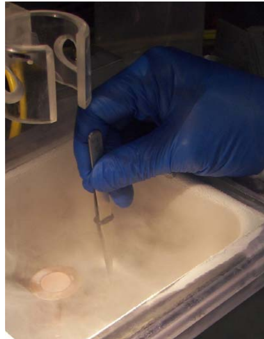
transfer of EM grid into cryo-storage box
