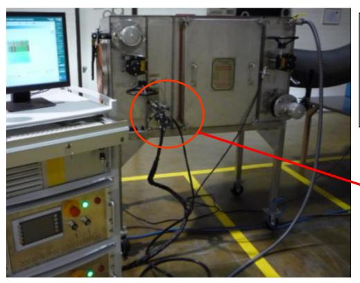
Housing connected to Filter Scanning Equipment via Tubes For "Hot Testing" we must decontaminate test equipment after scanning using special ports
