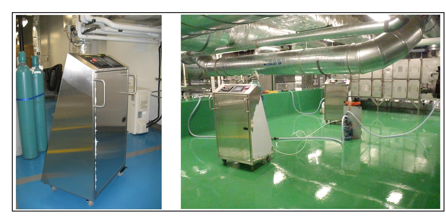
Figure 2. ClorDiSys Minidox-M Decontamination Unit and external blower set-up.
