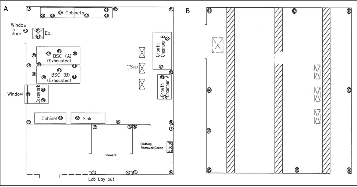
Figure 7. Typical room schematic of BI and CI placement in a BSL-3 lab during cycle optimization. The figure on the left shows BI and CI placement in the room (A). The figure on the right shows BI and CI placement above the false ceiling (B)
