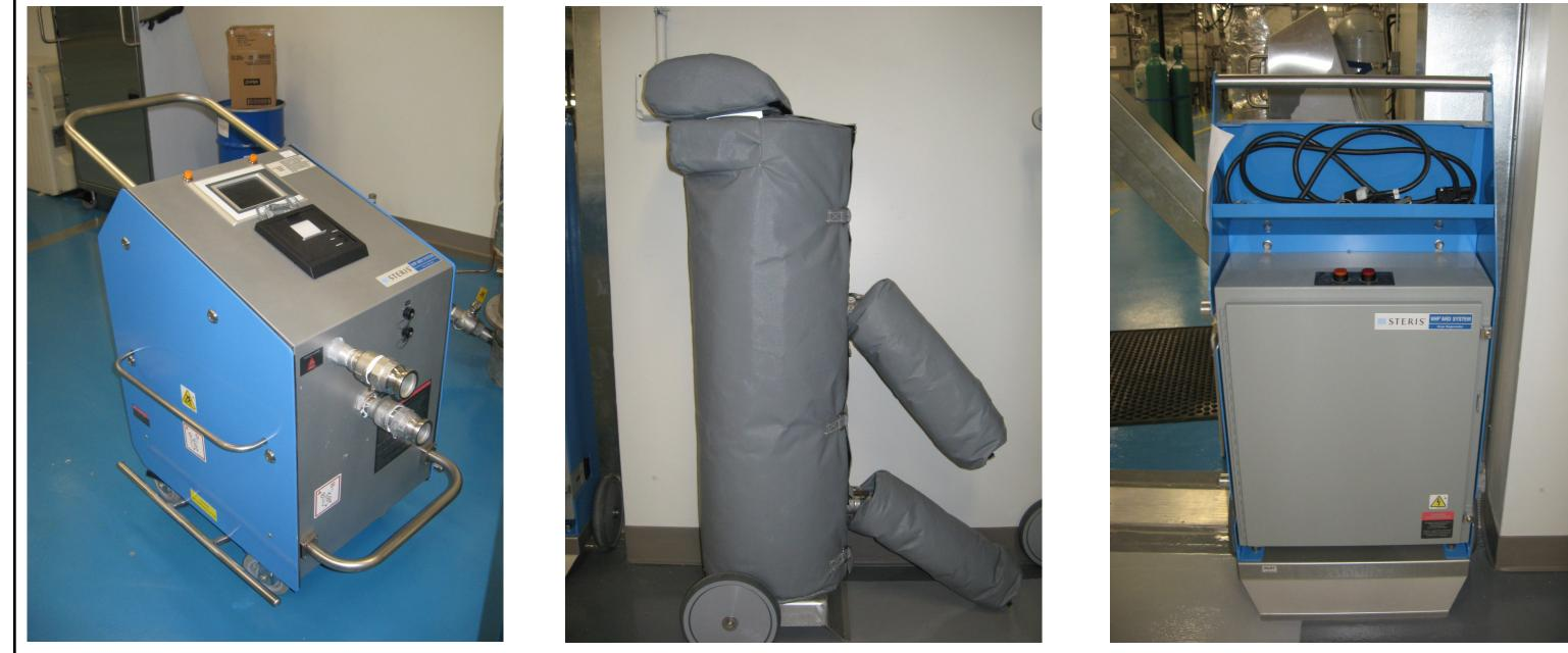
Figure 1. Steris VHP 1000-ARD System with dryer unit and dryer regeneration unit.
