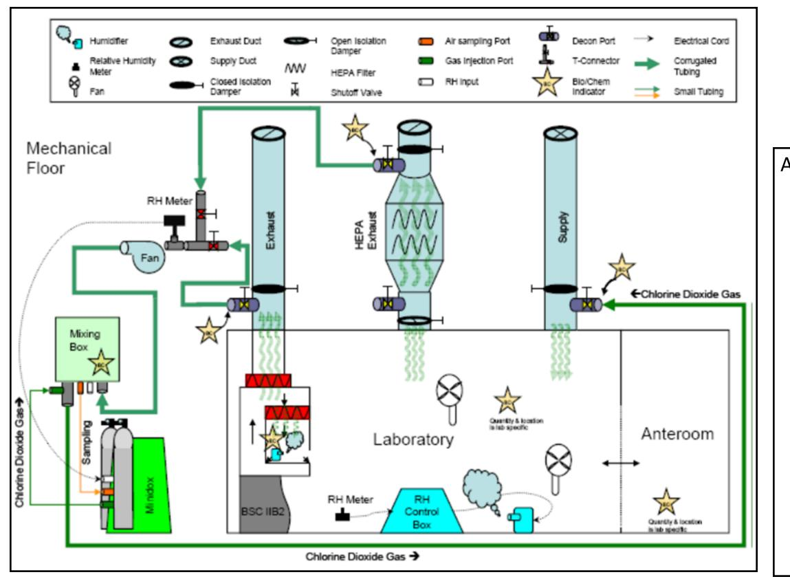
Figure 3. Closed loop system used at BRI (CD gas set-up shown).
