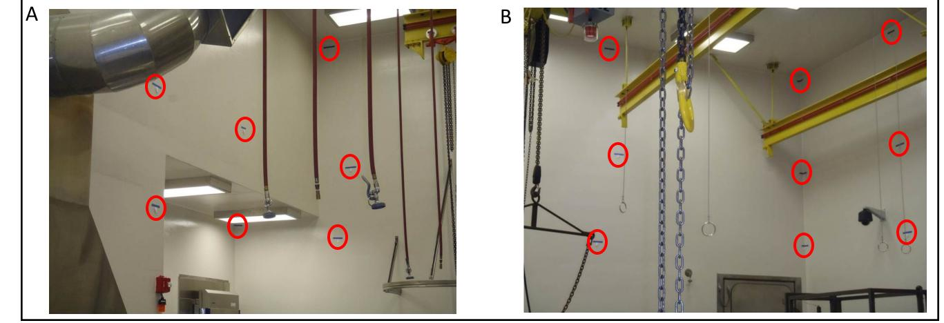
Figure 6. Biological (BI) and chemical (CI) indicator pairs hung throughout the room with blue painter's tape. During cycle optimization, BI and CI pairs are hung in predetermined spots throughout the room and in any hard-to-reach places
