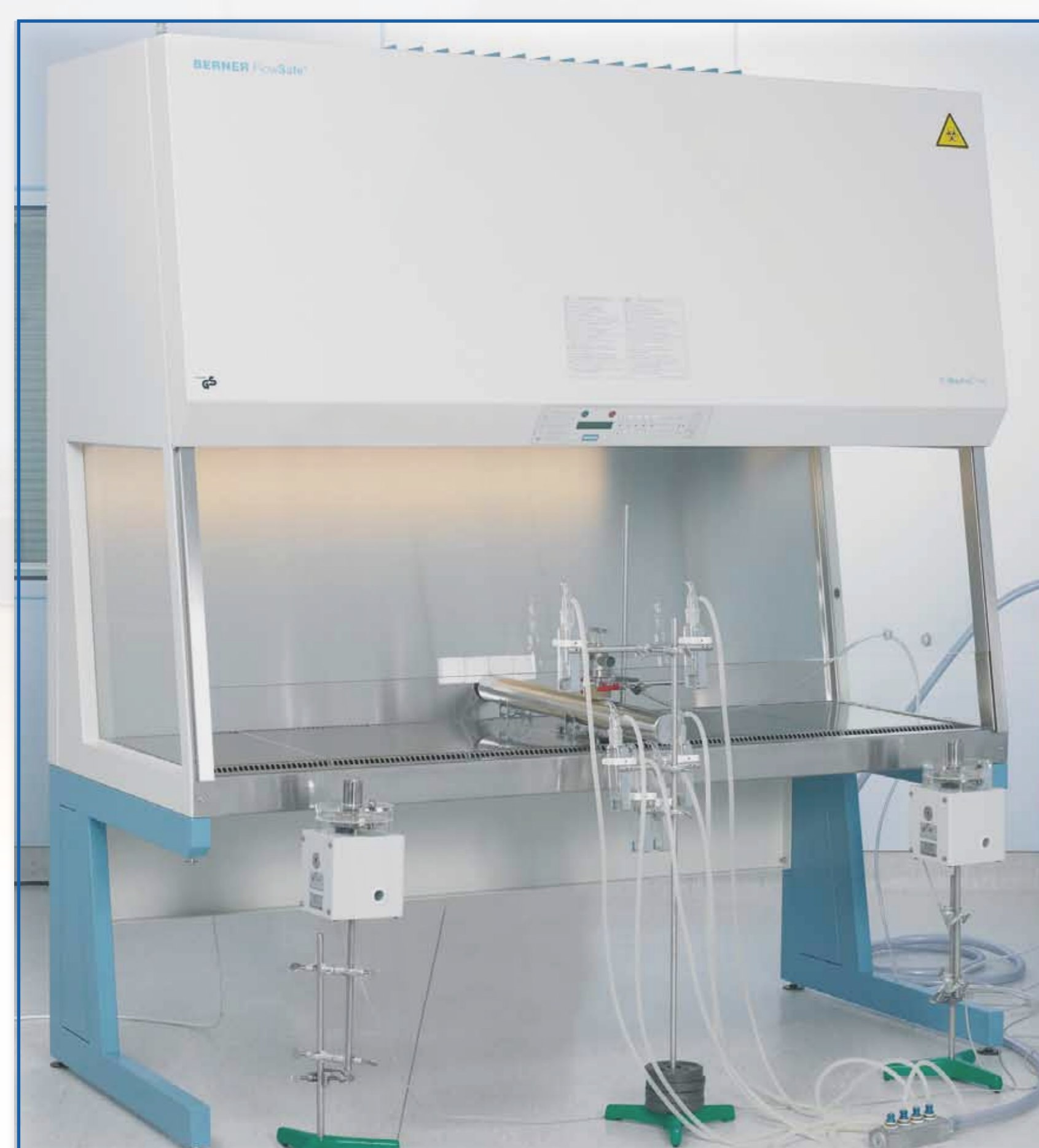
Fig. 1: Microbiological testing of personal protection based on EN 12469.
