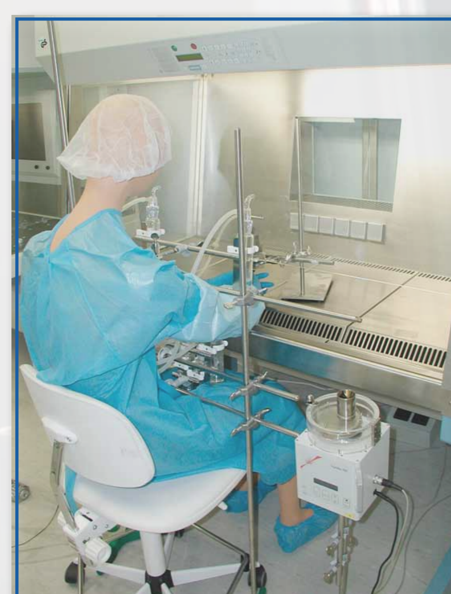
Fig. 2: Static interference „Person in front of SC“.
