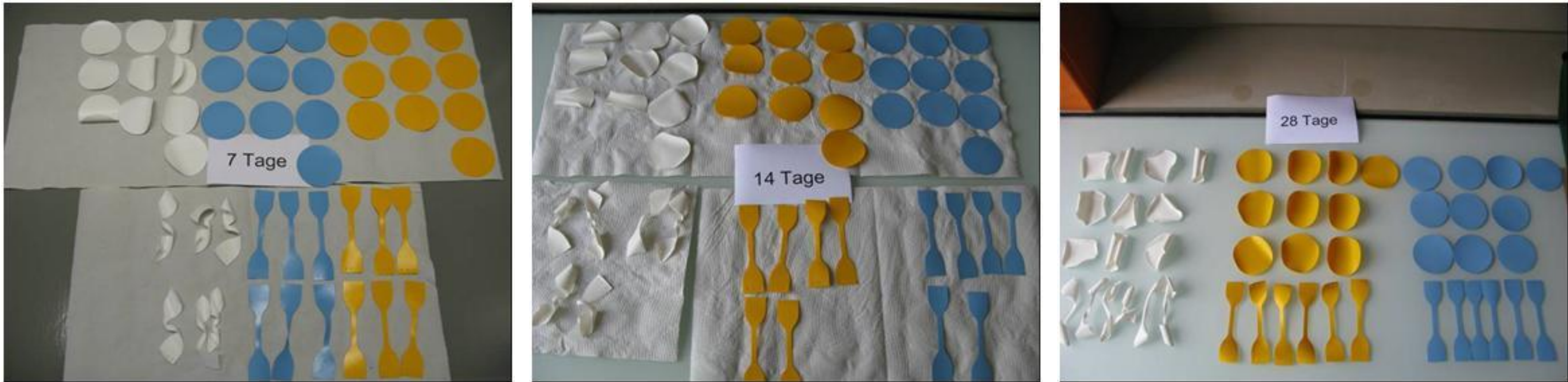
Fig. 2: Material Compatibility towards 2.5% Per-Acetic Acid BSL4 suit laboratories require a chemical shower process when leaving the laboratory. At the new facility at SPIEZ LABORATORY decontamination in the chemical shower is performed using per-acetic acid at a maximum concentration of 2.5%. A number of standard tests were performed in order to gain some insights into the material properties (data not shown). Material samples were immersed in 2.5% per-acetic acid for 7, 14 and 28 days and changes in the performance noted in comparison to non-incubated samples. Visually, differences in material compatibility could be clearly demonstrated with the blue suit giving the best results, followed by the yellow suit and finally the white one. Measurement results obtained from tensile, tear resistance and puncture tests, however, revealed that the yellow suit's material proofed to be best suited for exposure to per-acetic acid, followed by the blue suit. Throughout the tests, the white suit showed the lowest performance (data not shown).
