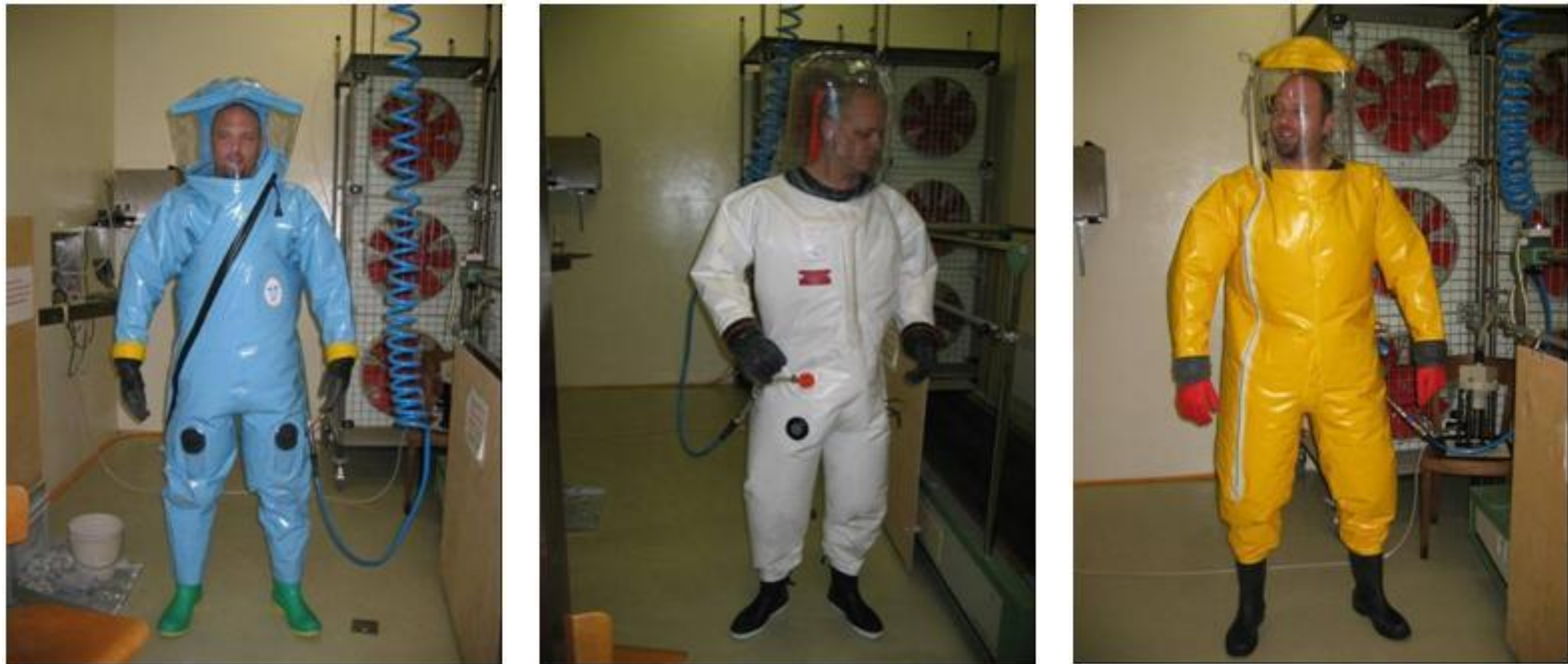
Fig. 1: Suit Models Used in the Study and Tests Performed Three suits by different manufacturers were tested. The suits will be differentiated by their colours (i. e. blue, white and yellow) and not their manufacturers' names. Tests in the following areas were performed: • Material compatibility: performance in 2.5% per-acetic acid • Protection factor: leak tightness (data not shown) and chemical protection factors • Wearer comfort: user feedback (data not shown).
