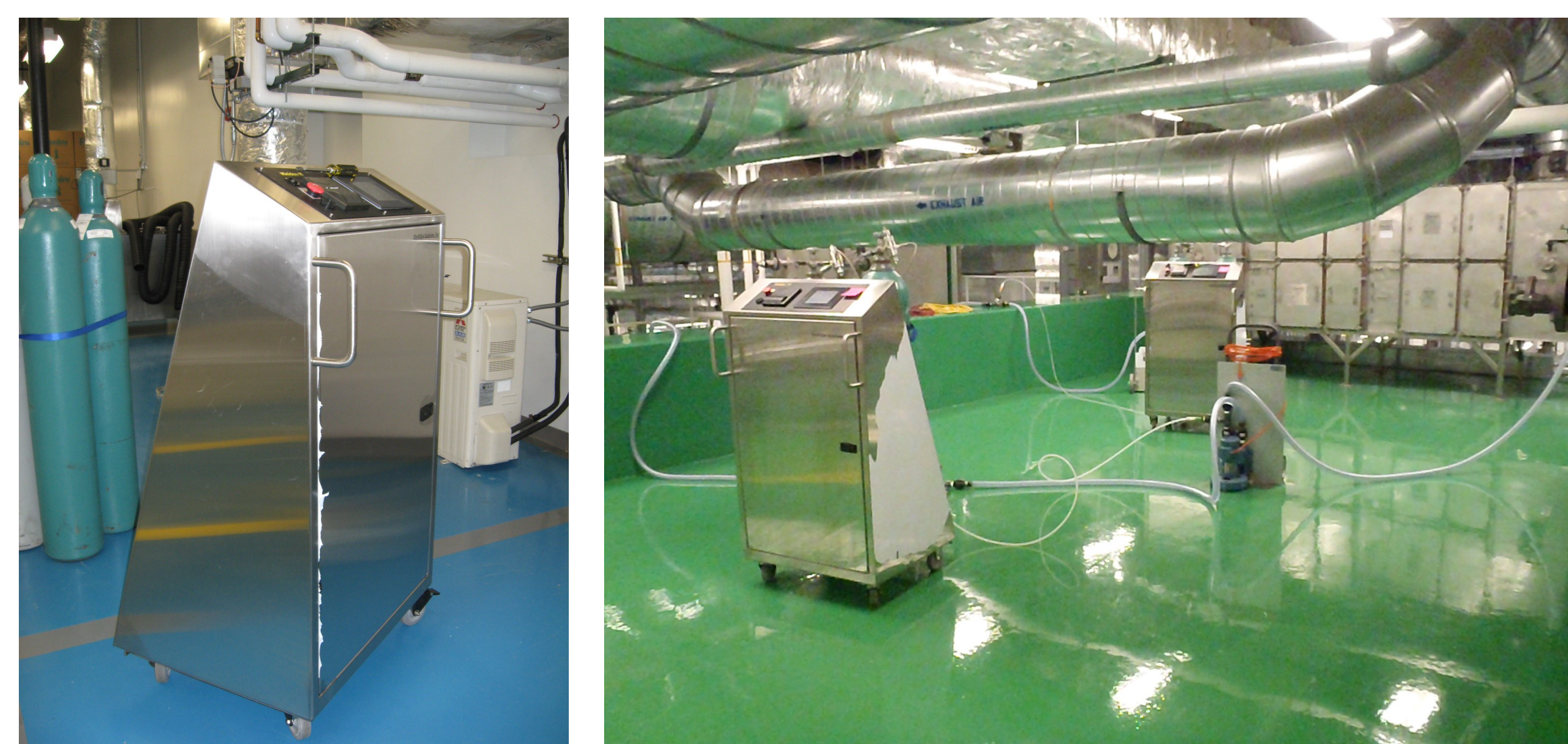
Figure 3. ClorDiSys Minidox-M Decontamination Unit and external blower set-up.
