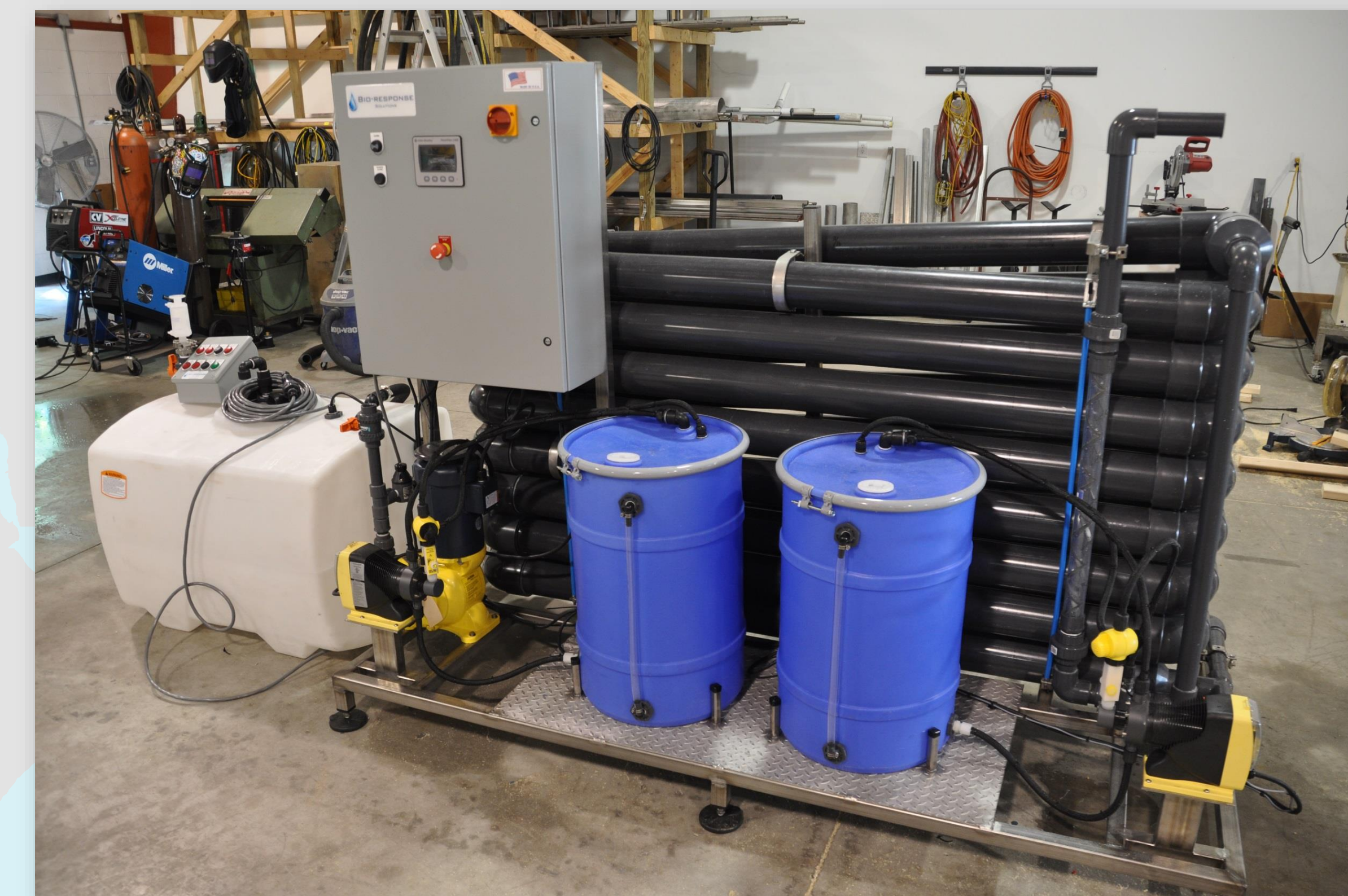
Batch Chemical EDS, 300 gallons per hour, $5 per hour ops cost, low capital cost
