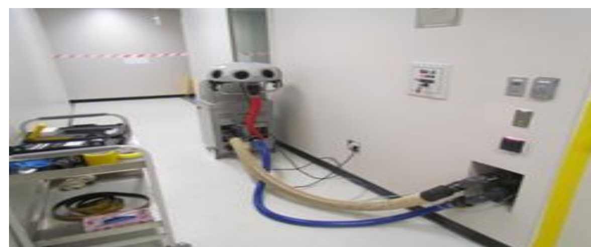
Figure 1. Bioquell Clarus L2 VHP decontamination unit at LC.
