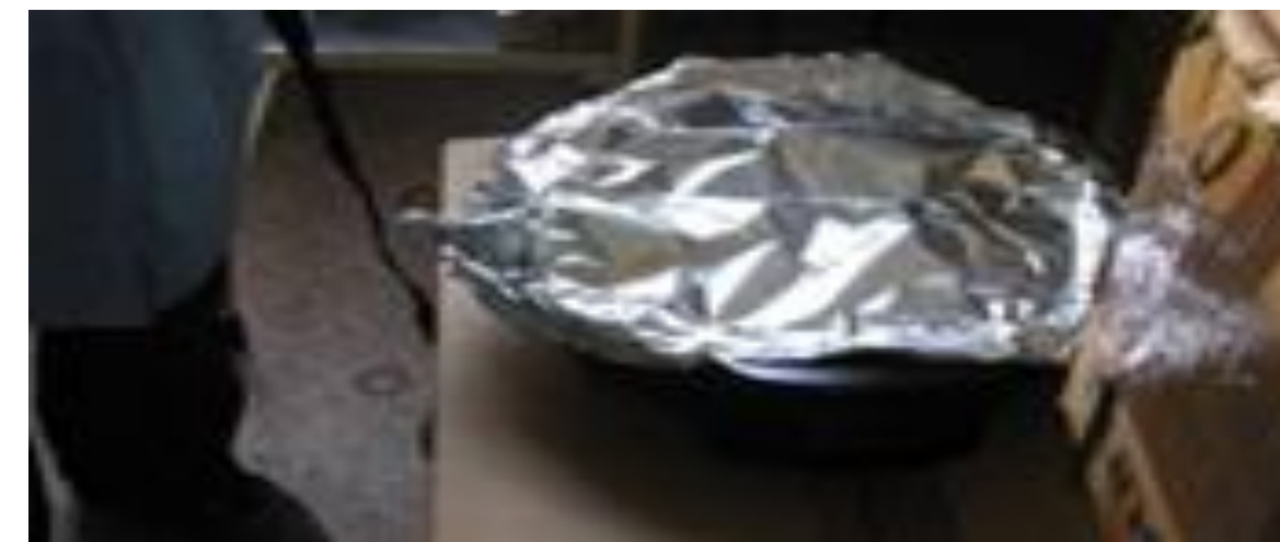
Figure 5. Ammonium bicarbonate covered with aluminum foil to prevent early neutralization.
