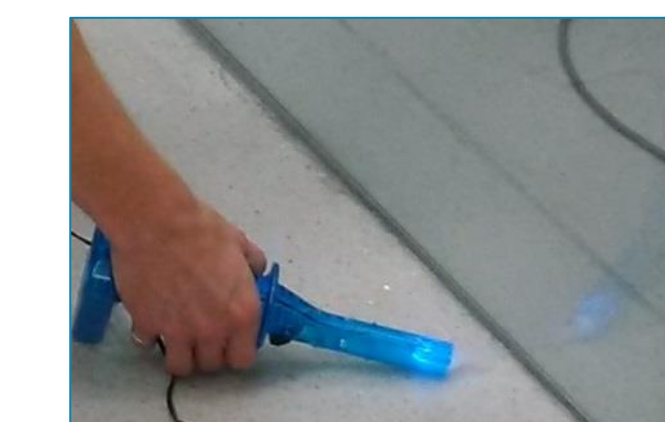
Figure 5. Smoke pencil demonstrating inward direction airflow when room in decontamination mode setting
