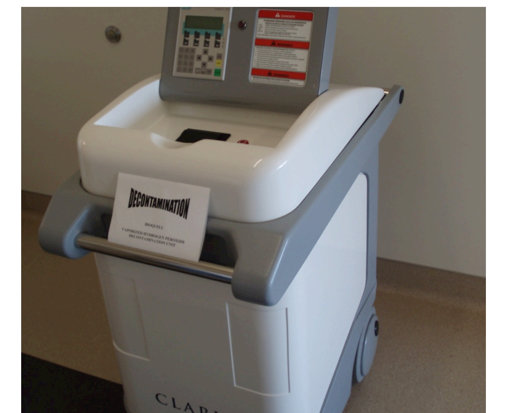
Portable VHP Sterilizer 30 to 35% hydrogen peroxide is delivered as vapor for surface sterilization.
