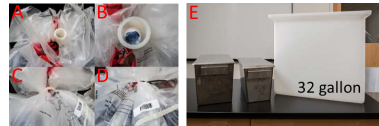
Figure 6. Examples of correct BagPipe usage (A-D) with an unobstructed opening (B) and autoclave pan options (E). From left to right the pans are 0.86 ft 3 (6.5 gallon), 0.51 ft 3 (3.8 gallon), and 4.3 ft 3 (32 gallon).
