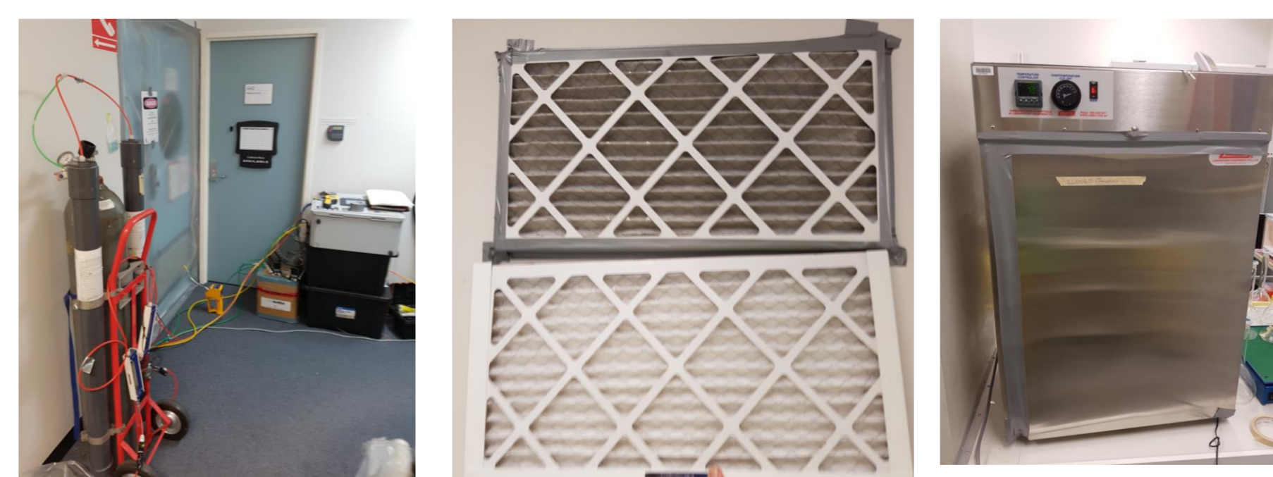
Figure 1.3 – The Cell culture laboratory after setup for fumigation had been completed. The air filter fitted on the supply air can be seen in the centre with the filter after 1 week operation. The sealed incubator containing live cultures can be seen on the left.
