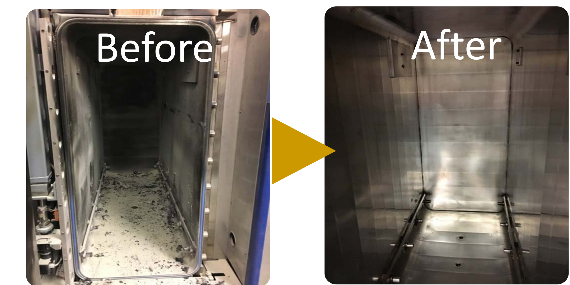
Figure 3. Autoclave before and after repairs/restoration
