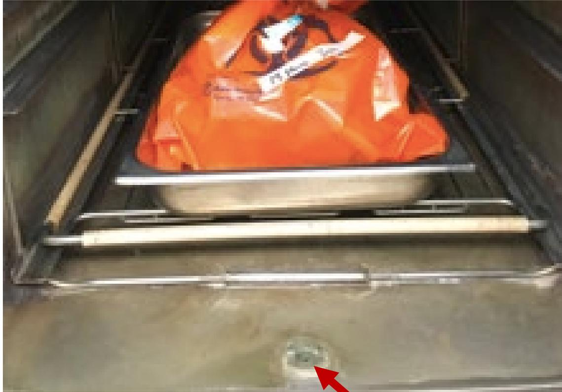
Check the drain and make sure it is clear – no debris or dried media
