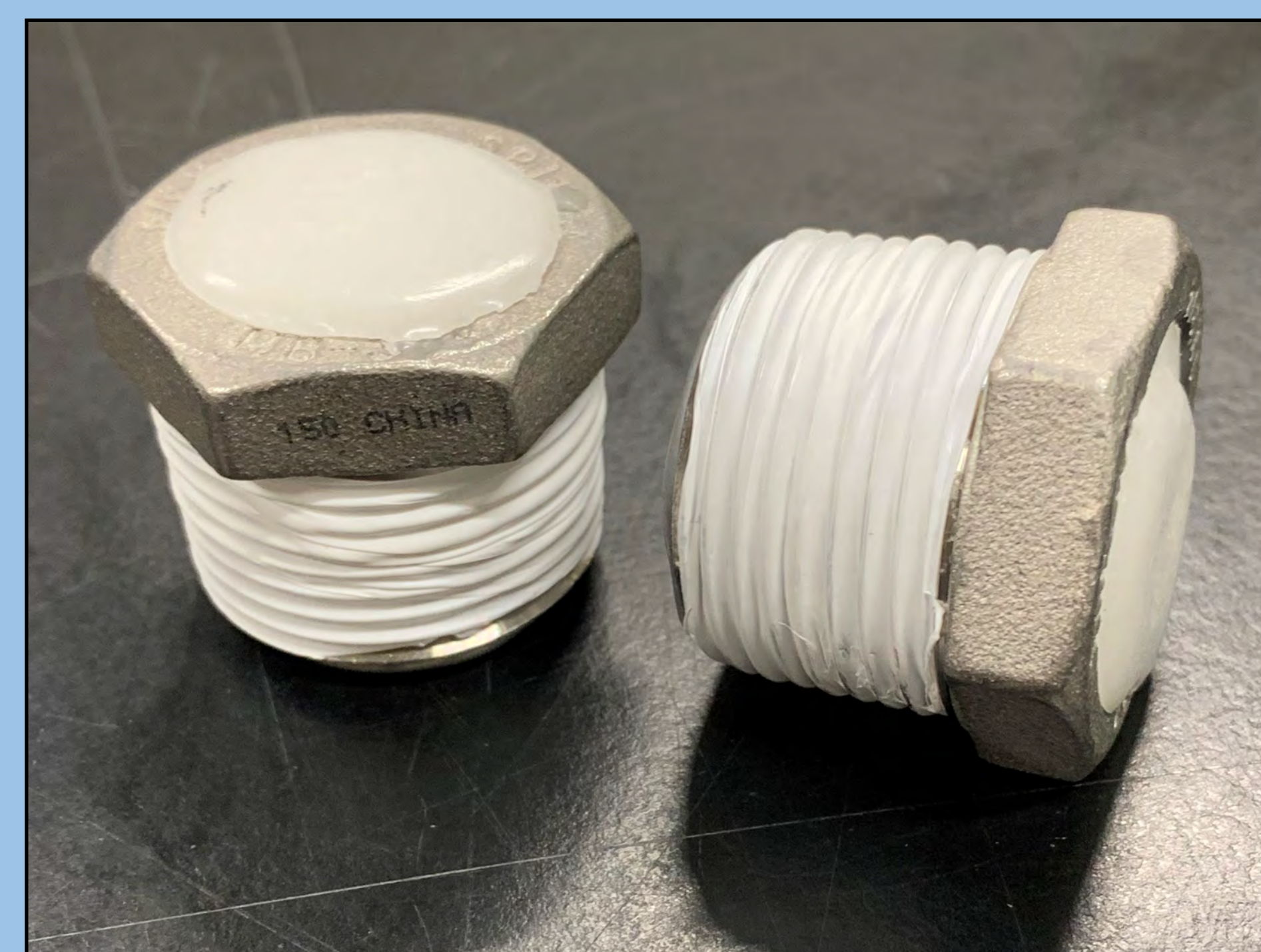
Paraffin wax plugs with threads wrapped in Teflon tape are designed to temporarily seal the MTC at room temperature until the melt point, ~100-150°F (~37-66°C), is reached during the autoclave cycle. The plugs are reusable when refilled with paraffin wax.
