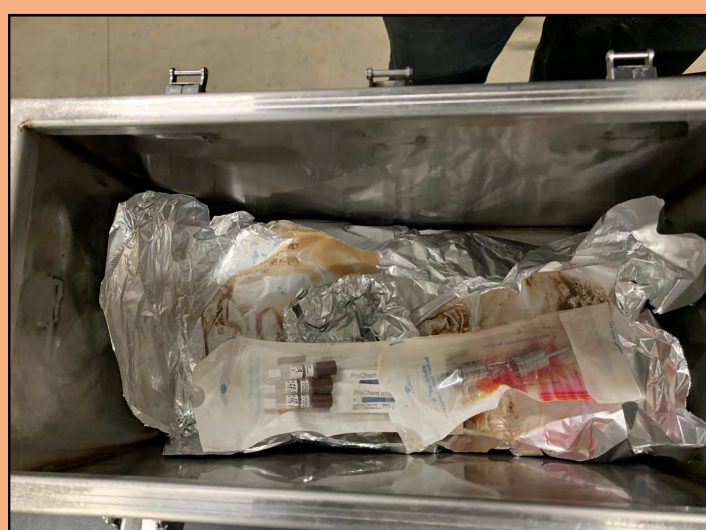
A MTC for the initial melt test contained an autoclave pouch with 3 SCBIs as well as a pouch with 2 data-loggers.
