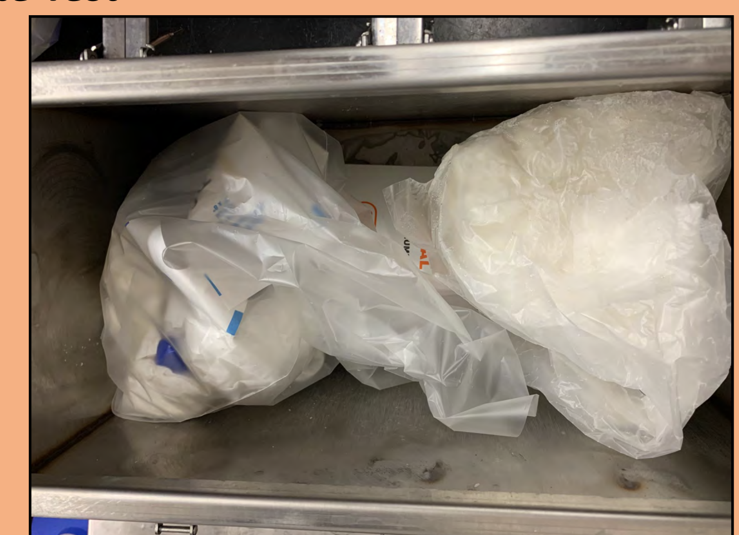
Representative mock laboratory waste used to obtain a thermal profile. The "hanger" bag also contained an autoclave pouch with 3 SCBIs and a pouch with 2 data-loggers.
