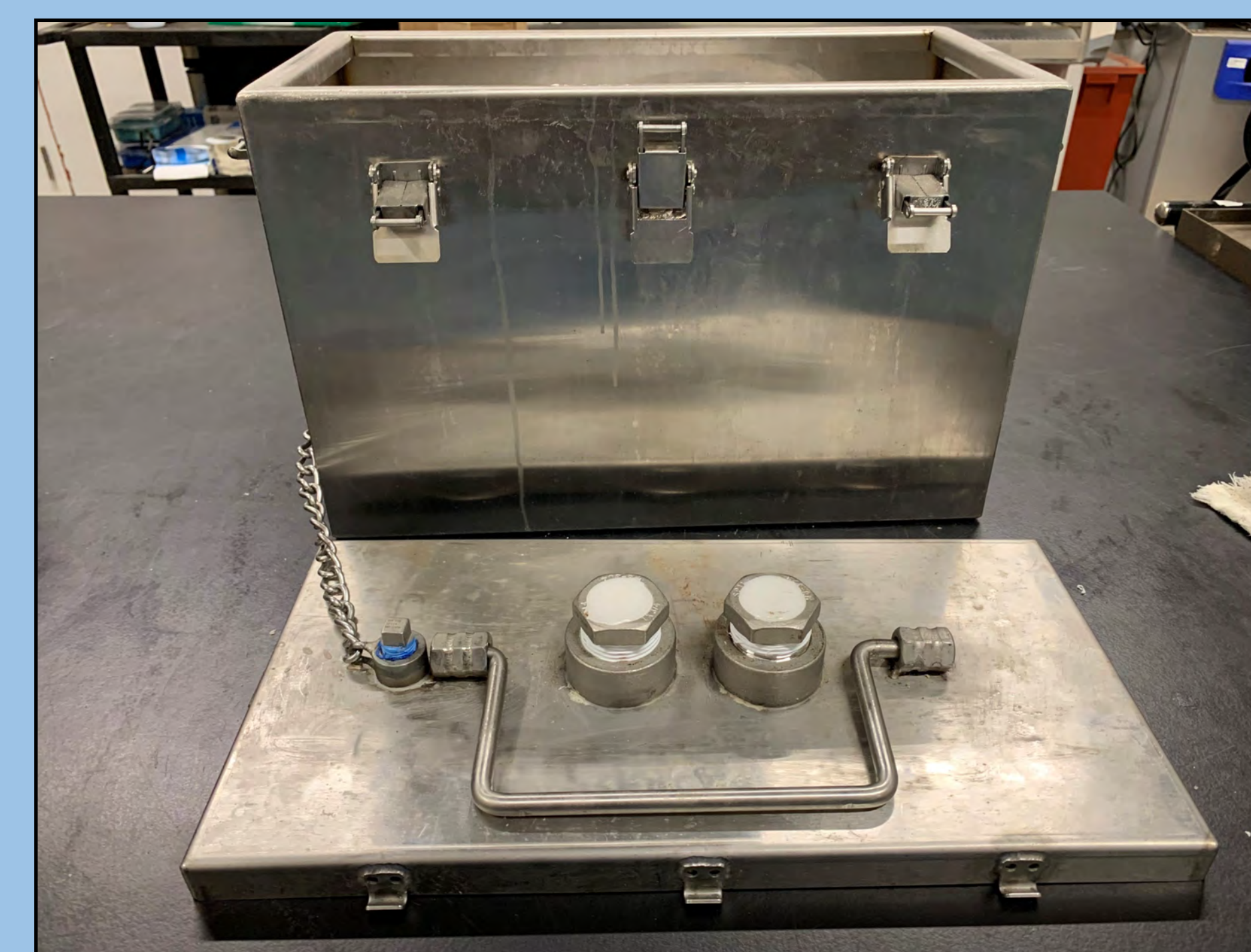
MTC with two threaded openings for reusable paraffin wax plugs to be inserted. The MTC is able to be closed and form an airtight seal (verified via pressure testing).
