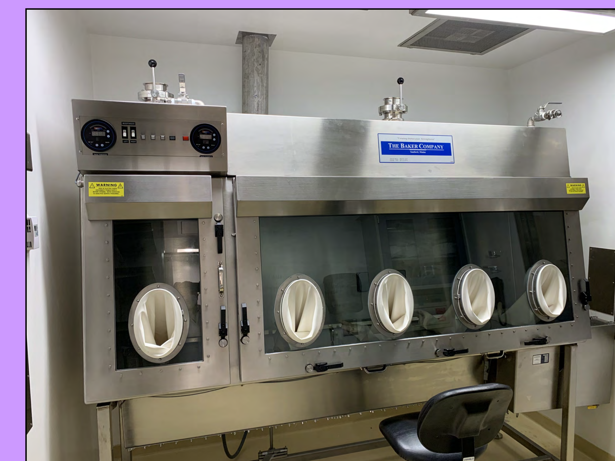
A Class III Biosafety Cabinet is designed to keep its contents completely sealed from the external environment. When an integrated autoclave is not possible, a modified transfer case can be used to contain any waste materials until the cabinet interior has been decontaminated and the transfer case has been removed and autoclaved.
