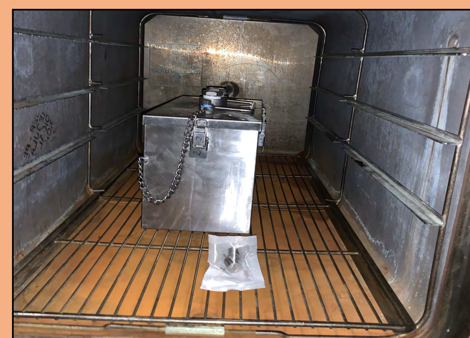
The MTC was placed inside the autoclave alongside an autoclave pouch containing 2 data-loggers to baseline chamber temperature.
